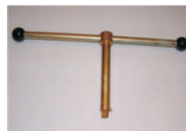
The handles for earthing switch control
