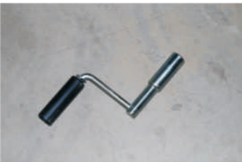
The crank-handle for the draw-out element control
